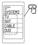
The selected component name is displayed on the bottom of the LCD display, and the labels for the operation of the component are displayed. To change the labels, press the SCROLL button repeatedly.
